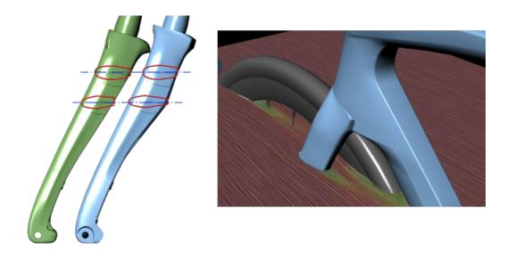
In the image the difference in the longitudinal section of the F12 fork (light blue) with respect to the F10(green) is visible. This increased section allowed better air channeling and reduced turbulence behind the fork.
