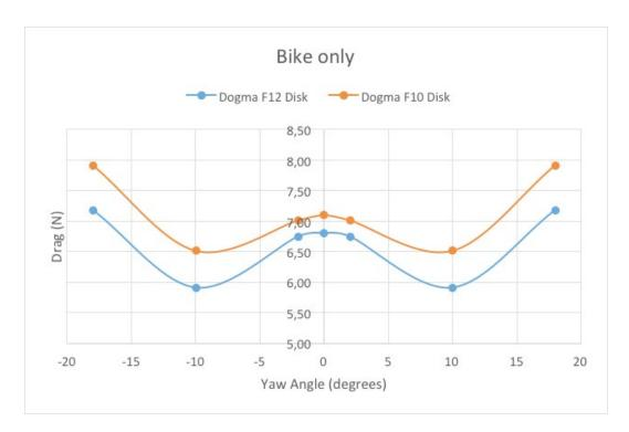
The graph shows the drag value at different yaw angles between the Dogma F12 Disk and F10 Disk. This study was just the bike itself. On average there is an improvement in aerodynamic efficiency by 7.3%. The improvement is even more effective when increasing the yaw angle (lateral wind).
