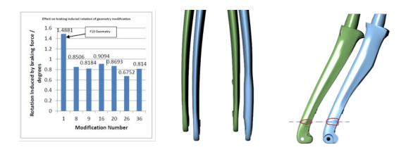
The right chainstay has been designed following the same principles. The shape is not straight, nor parallel to the right one, in fact it is dropped down and then shaped upwards nearby the rear caliper connection. This shape, also studied with FEM, guarantees a reduced deformation of the chainstay under the stresses coming from braking power.
