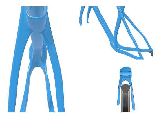
The frame is compatible with 12mmx100mm through axle on the front and 12mmx142mm axle on the rear. This offers the most complete range of compatibility with rims on the market both for road and MTB riding.
