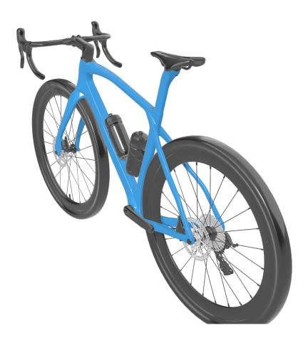
We wanted to keep the Q-factor similar to a road bike and without the need of lengthening the chainstay as to not affect the rideability. Therefore, it was necessary to move the chainstay downwards in order to free the critical intersection zone. This made it possible to guarantee a cross tube section of 14mm for chainstay, thus guaranteeing the optimal rigidity of the component.
