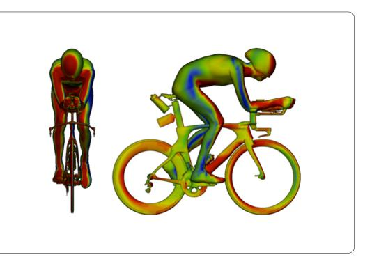
Once the initial parameters and the boundary conditions were defined, the aerodynamic study was carried out by breaking down the individual components of the Frame (as shown on the picture below) and evaluating their specific aerodynamic influence. Each element has therefore been optimized individually and then re-evaluated on the frame with an athlete present.
