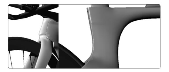
3 - REAR MONOSTAY. The advantage of mounting disc brakes allowed us to revise and optimized the monostay. In fact we completely removed the rim brake integration cover. So the monostay has been redesigned in such a way as to minimize its front surface and ensure an optimal air flow through to the rear wheel.
