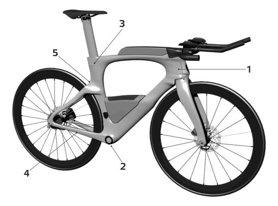
1 - HEADT TUBE: increased by 35mm compared to the Bolide TT. This allows for improved ergonomics and to have a more relaxed position on the bike without sacrificing aerodynamics. Combined with the Aero TT bar and the ability to add 40mm spacers under the extension + 10mm spacers under the pads, every rider can find their best position or adapt the position specific to the race type.
