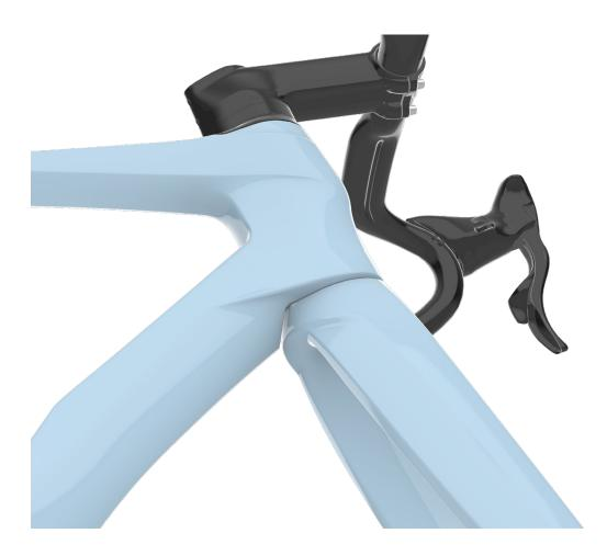
The introduction of "TiCR" implies to introduce the 1" ½ bearing both to the upper than lower side. Hence, we consequently enlarged the head tube, especially in the area near the top tube. This extra space allowed us to redesign the cross section with a more efficient aerodynamic shape than the previous MY20 Prince, as is illustrated below:
