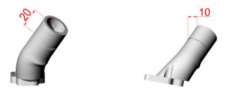
The handrips can be shortened up to the minimum mark located 20mm from the tip. The maximum reduction involves a shortening of the reach by 10mm.
