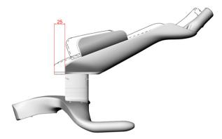
Continuous translation of the extensions is allowed up to a maximum of 25mm. The difference in reach gained based on the inclination of the extensions is negligible.
