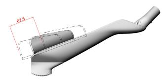
The position of the pads can vary along the direction of development of the extensions in steps of 11.25mm up to a maximum of 67.5mm between the two limit positions.
