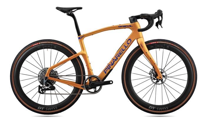
1. HEADTUBE AND SEATTUBE ANGLES: The geometry of the frame is specially designed to offer maximum comfort and performance on rough terrain. The angles of the seattube and headtube have been designed to ensure a position in the saddle that allows perfect control and comfort on the bike over long distances. Developed to allow you to keep power on the pedals even over rough terrain, the geometry enables you to get the most speed out of your effort deep into ultra-endurance events.
