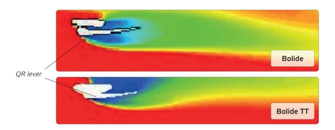
Images above show the comparison between slipstream generated by the left dropout and QR lever on Bolide and Bolide TT. What appears is that on Bolide TT, because of the design of the dropout which "encloses" part of the QR lever, the slipstream is narrower and, especially, tends to move towards the frame. On the contrary, on the Bolide, the slipstream moves away from the frame. So, even if locally the blue area is larger on Bolide TT, the gait of the slipstream lead to a lower final drag.
