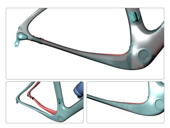
Another part of the frame that is heavily asymmetric is the top tube. The main reason for this as mentioned is to better accommodate the rider's shoulder. The other reason for designing the top tube in this way, was to address the aforementioned concept to enhance the asymmetry of this tube. Doing this the top tube's section is evidently unbalanced towards the right side of the bike. The result is again a better compensation of the asymmetrical forces that take place in the frame during riding.
