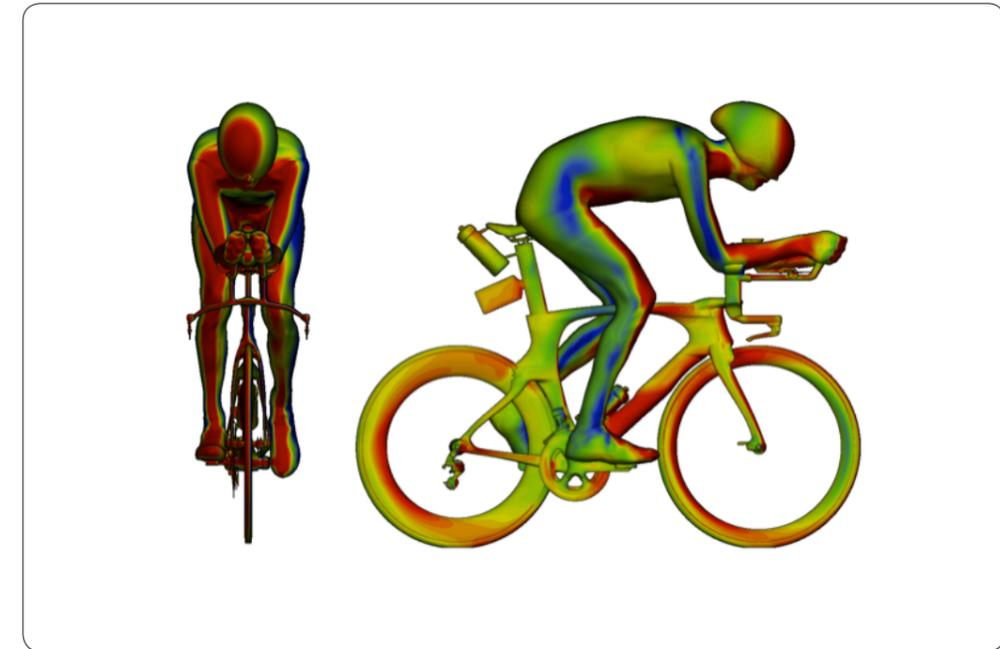
Once the initial parameters and the boundary conditions were defined, the aerodynamic study was carried out by breaking down the individual components of the Frame (as shown on the picture below) and evaluating their specific aerodynamic influence. Each element has therefore been optimized individually and then re-evaluated on the frame with an athlete present.
