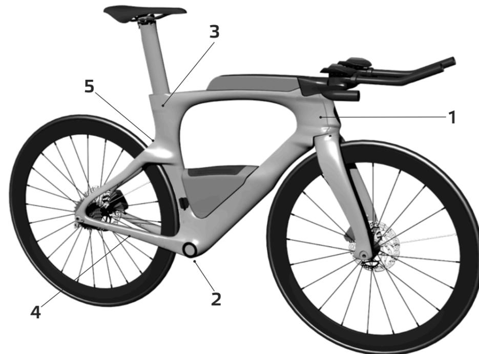
**1 - HEAD TUBE:** increased by 35mm compared to the Bolide TT. This allows for improved ergonomics and to have a more relaxed position on the bike without sacrificing aerodynamics. Combined with the Aero TT bar and the ability to add 40mm spacers under the extension + 10mm spacers under the pads, every rider can find their best position or adapt the position specific to the race type. Having a bigger head tube increases the rigidity of the bike frame and the overall stability of the head set.
