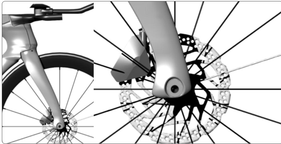
**2 - FRONT COVER.** The cable routing is completely integrated into the frame. The front cover, hides the routing of the front brake hose and is integrated with the fork. This guarantees aerodynamic improvements both with the surface between the cover and the fork being continuous, and the hosing is concealed from air flow.
